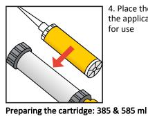
4. Place the cartridge into the application gun ready for use
