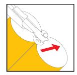
2. Cut the two plugs of the cartridge
